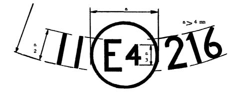
The approval number must be placed close to the circle surrounding the letter "E", but may be in any position with respect to it. The figures of the approval number must face the same way as the "E". The Roman numerals indicating the class must be diametrically opposite to the approval number. The competent authorities will avoid using approval numbers 1, 11 and 111, which might be confused with the class symbols I, II and III.
