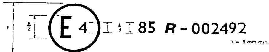
The above approval mark affixed to an engine shows that the engine type concerned has been approved in the Netherlands (E 4) with regard to the measurement of the net power, pursuant to Regulation No. 85 and under the approval number 002492. The approval number indicates that the approval was granted in accordance with the requirements of Regulation No. 85 in its original form.
