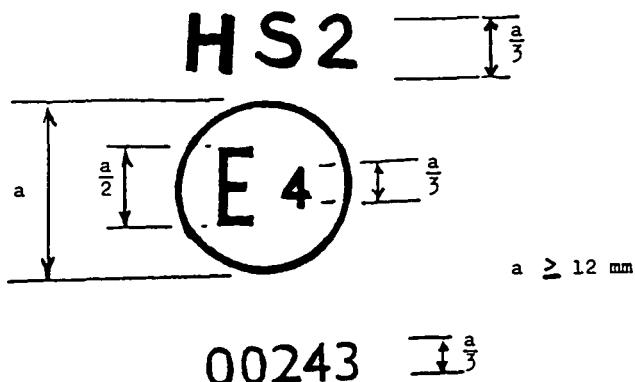
The headlamp bearing the above approval mark has been approved in the Netherlands (E 4) pursuant to Regulation No. 82 under approval number 00243. The first two digits of the approval number indicate that the approval was granted in accordance with the requirements of this Regulation in its original form.
