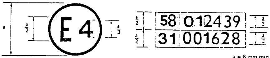
The above approval mark affixed to a vehicle shows that the vehicle type concerned has been approved in the Netherlands (E 4) pursuant to Regulations Nos. 58 and 31. 1/ The approval numbers indicate that, at the dates when the respective approvals were given, Regulation No. 58 included the 01 series of amendments and Regulation No. 31 was still in its original form.
