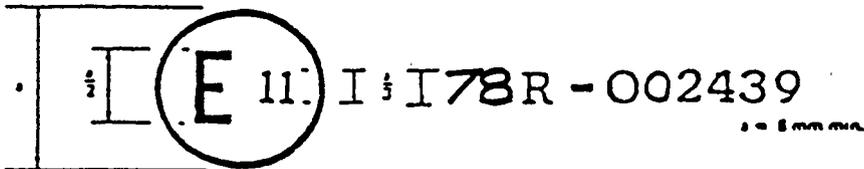
The above approval mark affixed to a vehicle shows that the vehicle type concerned has, with regard to braking, been approved in the United Kingdom (E 11) pursuant to Regulation No. 78 under approval number 002439. The first two digits of the approval number indicate that the approval was granted in accordance with the requirements of the Regulation in its original form.
