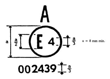
The above approval mark affixed to a special warning light indicates that it has been approved in the Netherlands (E 4), under approval number 002439. The approval number shows that approval was granted in accordance with the requirements of the Regulation in its original form and is a class "A" light.
