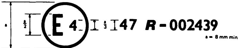
The above approval mark affixed to a vehicle shows that the vehicle type concerned has, with regard to the emission of gaseous pollutants by the engine, been approved in the Netherlands (E4), pursuant to Regulation No. 47. The approval number indicates that the approval was granted in accordance with the requirements of Regulation No. 47 in its original form.
