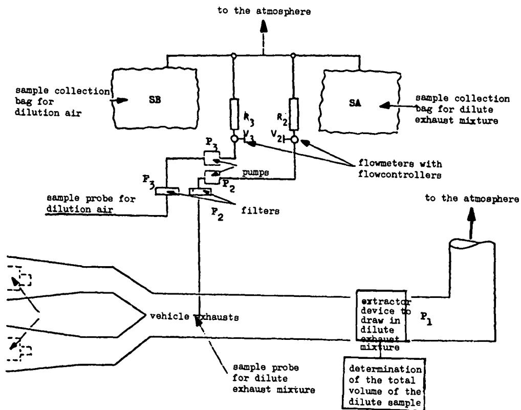
*Annex 4 – Appendix 4***METHOD FOR CALIBRATION OF THE DYNAMOMETER BENCH****1. SCOPE**
