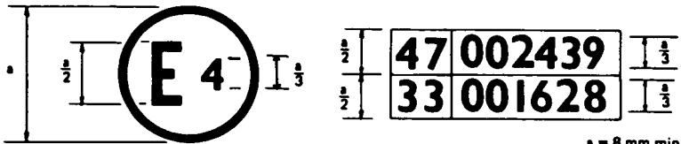
The above approval mark affixed to a vehicle shows that the vehicle type concerned has been approved in the Netherlands (E4) pursuant to Regulation No. 47 and Regulation No. 33.\* The approval numbers indicate that, at the dates when the respective approvals were given, Regulations Nos. 47 and 33 were still in their original form.
