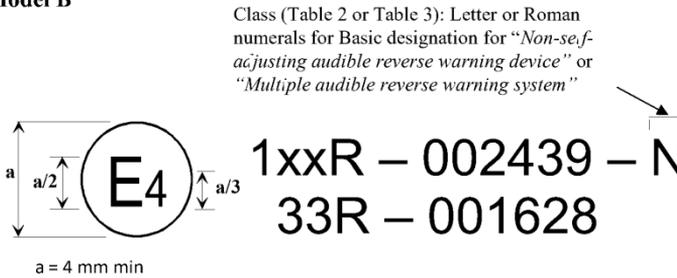
The above approval mark affixed to a vehicle shows that the vehicle type has device(s) of Class N and has been approved in the Netherlands (E 4) pursuant of UN Regulations No. [1xx] and 33.<sup>1</sup> The approval numbers indicate that, at the dates when the respective approvals were granted, UN Regulation No. [1xx] and UN Regulation No. 33 were in their original form.
