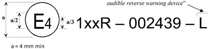
The above approval mark affixed to an audible reverse warning device of Class L shows that this audible reverse warning device has been approved in the Netherlands (E 4) under approval number 002439. The first two digits of the approval number indicate that the approval was granted in accordance with the requirements of UN Regulation No. [1xx] in its original form.
