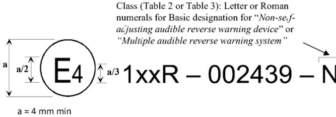
The above approval mark affixed to a vehicle indicates that, pursuant of UN Regulation No. 1xx, this vehicle type has device(s) of Class N and has been approved in the Netherlands (E 4), with regard to its audible warning signals. The first two digits of the approval number indicate that UN Regulation No. [1xx] was in its original form.
