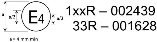
The above approval mark affixed to a vehicle shows that the vehicle type has been approved in the Netherlands (E 4) pursuant to UN Regulations Nos. [1xx] and 33.<sup>2</sup> The approval numbers indicate that, at the dates when the respective approvals were granted, UN Regulation No. [1xx] and UN Regulation No. 33 were in their original form.
