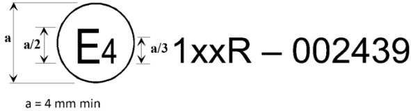
The above approval mark affixed to an audible reverse warning device shows that this audible reverse warning device has been approved in the Netherlands (E 4) under approval number 002439. The first two digits of the approval number indicate that the approval was granted in accordance with the requirements of UN Regulation No. [1xx] in its original form.
