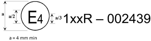
The above approval mark affixed to a vehicle indicates that, to UN Regulation No. [1xx], this vehicle type has been approved in the Netherlands (E 4), with regard to its audible warning signals. The first two digits of the approval number indicate that UN Regulation No. [1xx] was in its original form.
