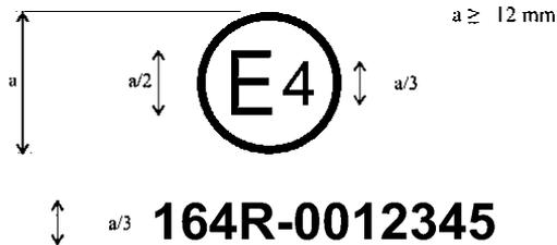
The above approval mark, affixed to a tyre shows that a tyre concerned has been approved in the Netherlands (E4) pursuant to UN Regulation No. [164], under approval number 0012345. The first two digits of the approval number (00) indicate that the approval was granted according to the requirements 00 series of amendments to this Regulation.
