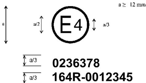
The above approval mark (according to paragraph 5.5. of this Regulation) shows that the tyre concerned has been approved in the Netherlands (E4) pursuant to UN Regulations Nos. 30 and [164]. The first two digits of the approval numbers indicate that, at the dates when the respective approvals were granted, UN Regulation No. 30 included the 02 series of amendments while UN Regulation No. [164] was in its original form.
